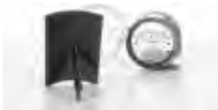
figure 13.3 Magnehelic Gauge with Air Flow Grid
